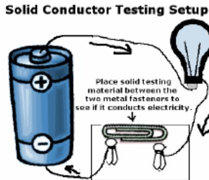
If the object makes the light bulb light up that means it completed (or closed) the circuit. This must mean that electrons can flow through it! If electrons can move easily through the materials, it is called a **conductor**.
