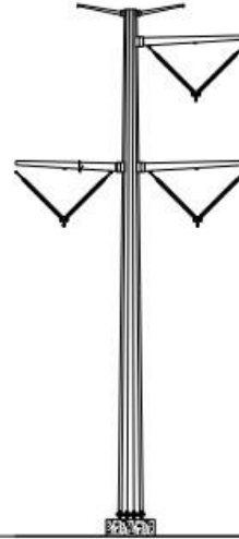
Monopole Tangent Delta 500kV Single Circuit Fdn. Width: Up to 20 ft. Height: Up to 190 ft.
