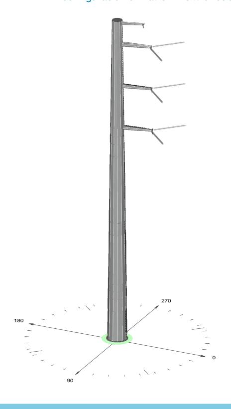
FIGURE G-12 Single-Circuit 230 kV Single-Pole, Dead-End, Delta
