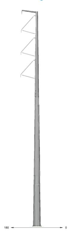
FIGURE G-3 Single-Circuit 230 kV Single-Pole, Tangent, Delta
