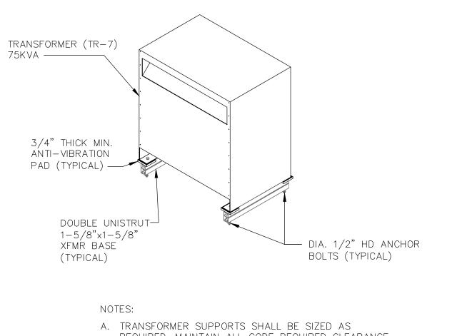
REQUIRED. MAINTAIN ALL CODE REQUIRED CLEARANCE AND MANUFACTURES SPECIFICATIONS.
