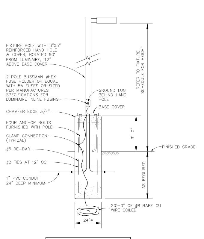
NOTE: THIS DETAIL IS SHOWN FOR ELECTRICAL INFORMATION ONLY. THE POLE/FIXTURE MANUFACTURER SHALL PROVIDE STRUCTURAL CALCULATIONS.
