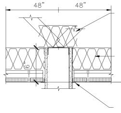
PROVIDE 3-5/8"x20 GA.STUD DIAG. BRACING AT 4'-0" O.C. TO STRUCTURE ABOVE FOR EVERY 8 LINEAL FEET OF WALLS UNSUPPORTED BY PERPENDICULAR WALLS. ALTERNATE DIAGONAL BRACING WHERE REQUIRED
