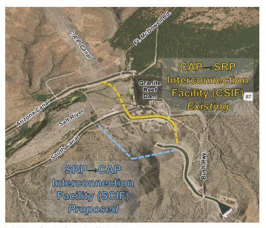
Jointly funded project to move non-project water stored in SRP reservoirs and underground storage facilities through the CAP canal
