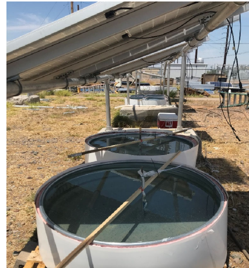
PV Panels + Evaporation Pans
